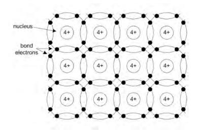
The outer shell of Silicon has 4 electrons in it. When silicon is in a crystalline state, the outer orbits share an electron with each other giving each atom 8 electrons in their respective outer orbits.
