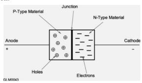
Because of the barrier region, the applied voltage must exceed 0.6V to 0.7V (0.2 to 0.3V for germanium diodes) in order to get current flow. When the voltage is attached negative to the N and positive to the P material, the negative voltage repels free electrons in the N material which are simultaneously being pulled toward the attractive positive charge on the P material—current flows and all is good.
