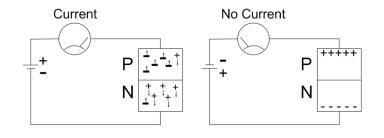
If instead the opposite voltage polarity is applied, negative to P and positive to N, then the positive side pulls all the free electrons to itself while the negative repels them. The result is that most of the diode becomes one giant depletion region and current cannot flow. The diode is said to be reverse biased. ®
