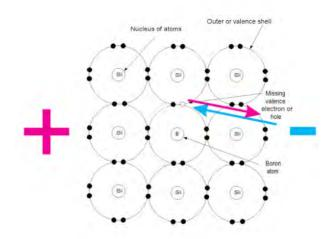
If instead we dope the silicon with gallium or boron, we then get a hole in the bond where the missing electron is. This is a P-type material.
