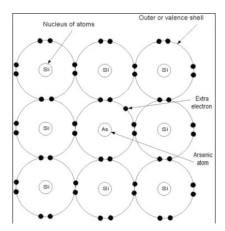
Here we see a crystal of silicon with arsenic atoms added. The extra electron in the outer shell of the arsenic atom is not used in the bond with neighboring silicon atoms and so is an extra, or *free*, electron. Because this crystal has an extra electron it is called the N-type material (*N* for negative) and if a voltage is applied that free electron is repelled by the negative charge and attracted to, and moves toward, the positive charge.
