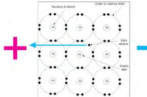
When these P- and N-type materials are joined together they form a junction between them. With no voltage applied the free electrons in the N material drift across the junction to fill the holes in the atoms nearby. This creates a depletion region, or a kind of no man's (no electrons) land at that interface between the materials. This PN junction is called a diode and it will only allow current to flow in one direction.
